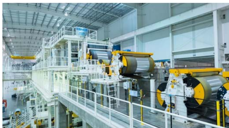
* CALP: Continuous Annealing Line with Pre-treatment
